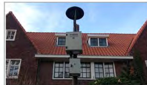
AirBox mounted on streetpole
